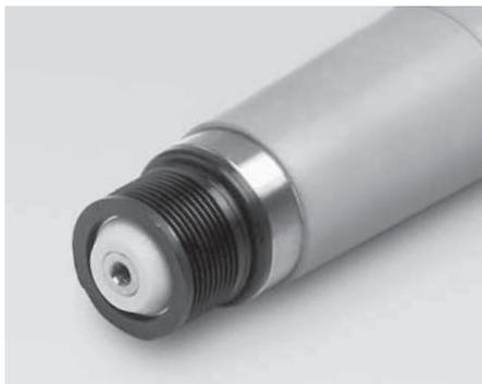
**RULLI CONICI COMANDATI CON PULEGGIA PER TRASMISSIONE CON CINGHIE FLESSIBILI POLY-V**
